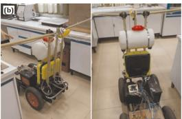
Another team of Iranian scientists has developed a prototype robot for precision planting of seeds in trays. A prototype seeder was designed with the help of the SolidWorks software, later it was tested for planting of tomato seeds. The seeder consists of several parts. The test results proved that the design capacity of the sowing robot is 17-35 thousand seeds per hour. Average precision of the developed system is 88%; design productivity of the system for sowing seeds is 170 trays per hour.
